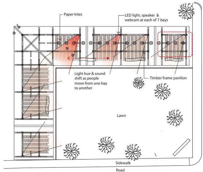
Figure 4: Site plan showing seven bays of the pavilion from which lanterns are hung. Each bay is equipped with an RGB LED fixture, webcam, and speakers.
